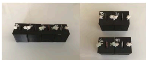
Figure 15. 3D-printed Low Cost half-cells for a pupil-centered experiment
