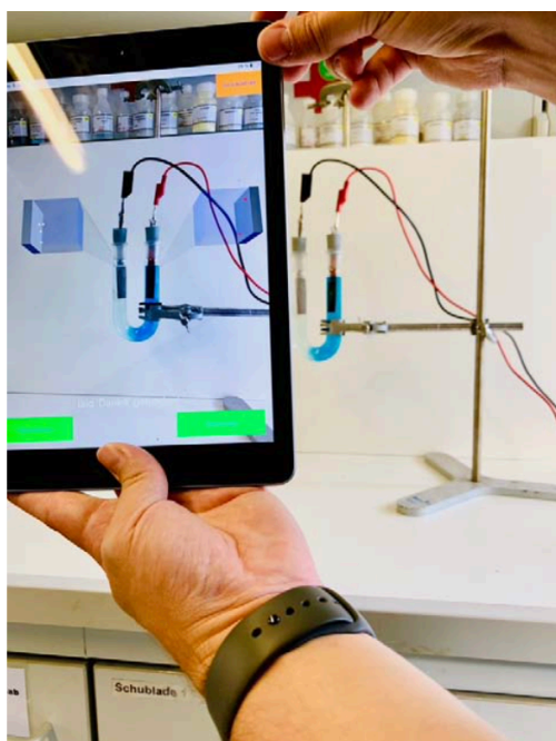
Figure 14. Augmented Reality of the microscopic level in a Daniell element
