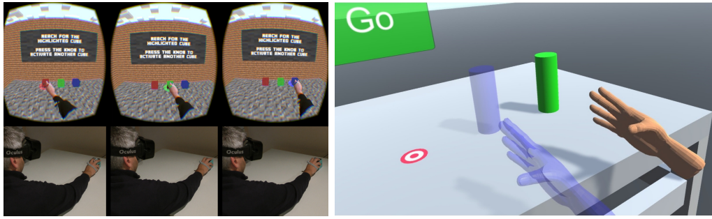
Figure 2.36: Two examples of haptic retargeting. Left: HR enabling a single proxy to provide haptic feedback for three displaced virtual cubes (extracted from [Azmandian et al., 2016b]; © 2016 ACM). Right: The real hand and proxy (blue) are offset from their virtual counterparts (colored) (extracted from [Han et al., 2018]; © 2018 IEEE).
