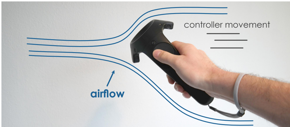
Figure 6.1: Drag:on leverages the airflow occurring during controller movements.
