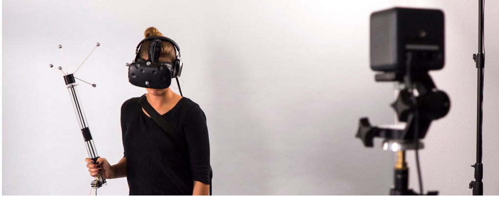
Figure 5.2: A user interacting with the DPHF proxy Shifty . Shifty can change its internal weight distribution to adapt its passive haptic feedback. By this, Shifty is designed to enhance the perception of virtual objects and their kinesthetic qualities. ©2017 IEEE.
