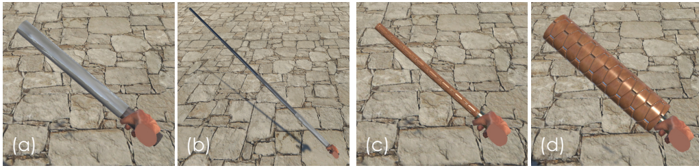
Figure 5.5: The objects of Experiment 1 changing in length and thickness: (a) the telescope object at 50cm length and (b) at 200cm length, (c) the rod-shaped object in the thinnest configuration and (d) in the thickest configuration. All images © 2017 IEEE.
