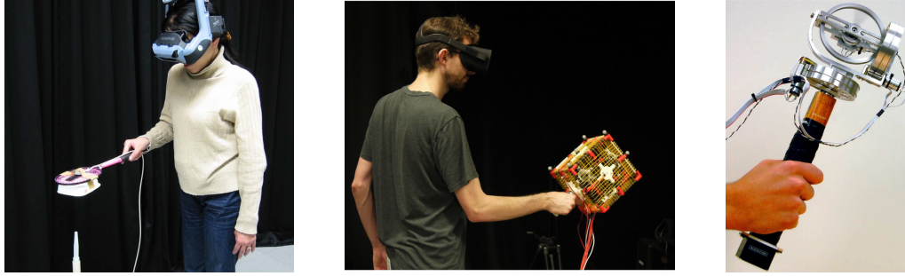
Figure 2.10: Three examples of ungrounded kinesthetic AHF. Left: A system releasing air from an air nozzle, which is felt through a handheld air receiver (extracted from [Suzuki et al., 2002]; © 2002 Suzuki and co-authors). Center: Thor's Hammer providing propeller-driven feedback (extracted from [Heo et al., 2018]; © 2018 Heo and co-authors). Right: iTorqU 2.0 torque feedback device (extracted from [Winfree et al., 2009]; © 2009 IEEE).
