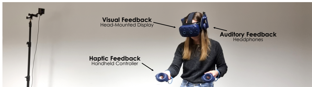
Figure 1.1: A typical VR system that conveys the look and sound of an Immersive Virtual Environment (IVE) through a Head-Mounted Display (HMD) and headphones. Interactions with virtual objects are performed by means of handheld VR controllers, which usually provide basic haptic feedback through vibration.
