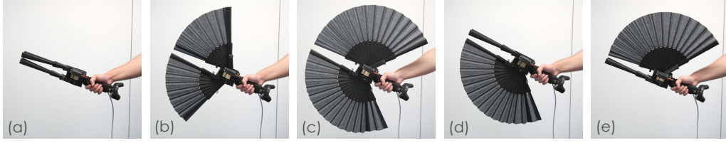
Figure 6.2: The five states of our shape-changing haptic VR controller Drag:on investigated in this chapter. (a) The device state S_{closed} with minimal surface area. When increasing its surface area symmetrically as shown in (b) ( S_{half} ) and (c) ( S_{full} ), the controller adapts its drag and mass distribution to provide different haptic sensations during VR interaction. If opened asymmetrically on the (d) left ( S_{left} ) or (e) right ( S_{right} ) side, torque is induced when moving the controller.
