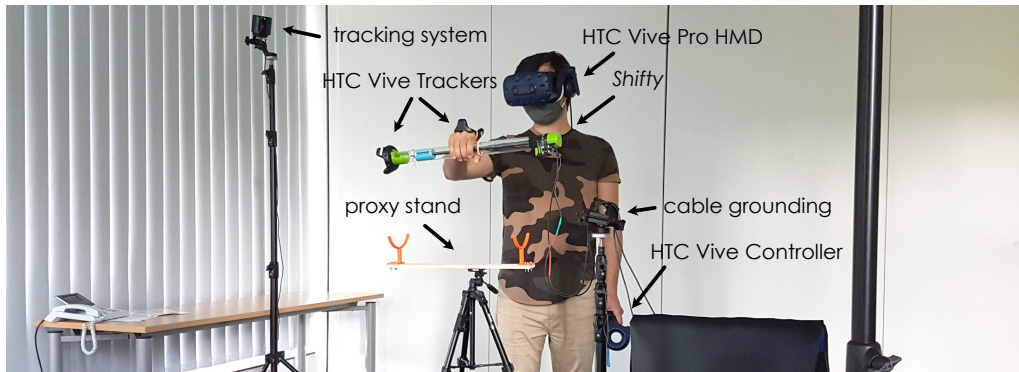
Figure 12.5: Experiment setup and involved components. The cable of the proxy has been grounded with a tripod to minimize gravitational pull. © 2021 IEEE.
