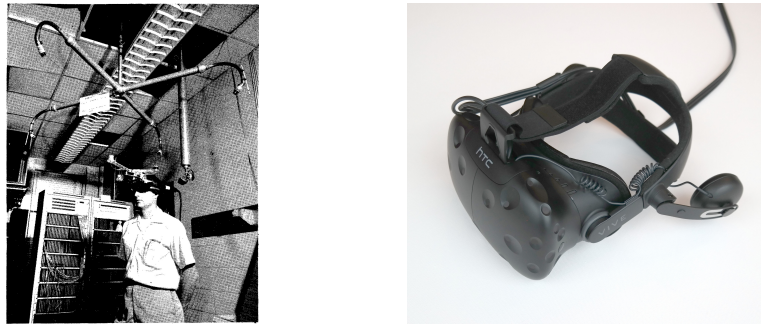
Figure 2.2: Left: The Sword of Damocles HMD of Sutherland (extracted from [Sutherland, 1968]; © 1968 ACM). Right: The HTC Vive – an example of a modern HMD.
