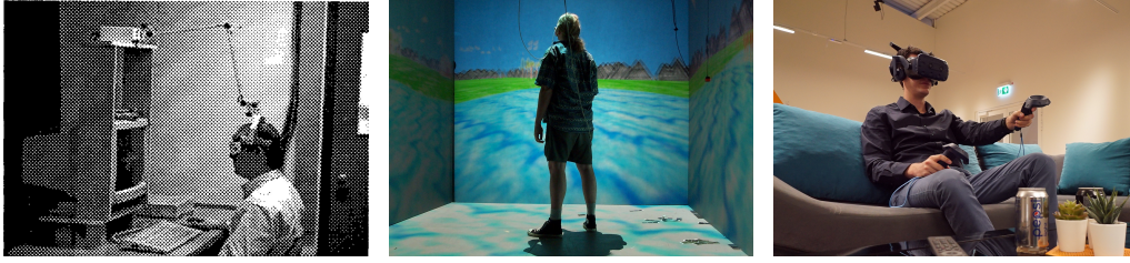
Figure 2.4: Left: Early implementation of Fish Tank VR (extracted from [Ware et al., 1993]; © 1993 ACM). Center: A user in a CAVE system experiencing projection-based VR (Source: Wikimedia Commons; public domain 13 ). Right: The author of this thesis wearing a wireless version of the HTC Vive Pro, a modern HMD-based VR system.
