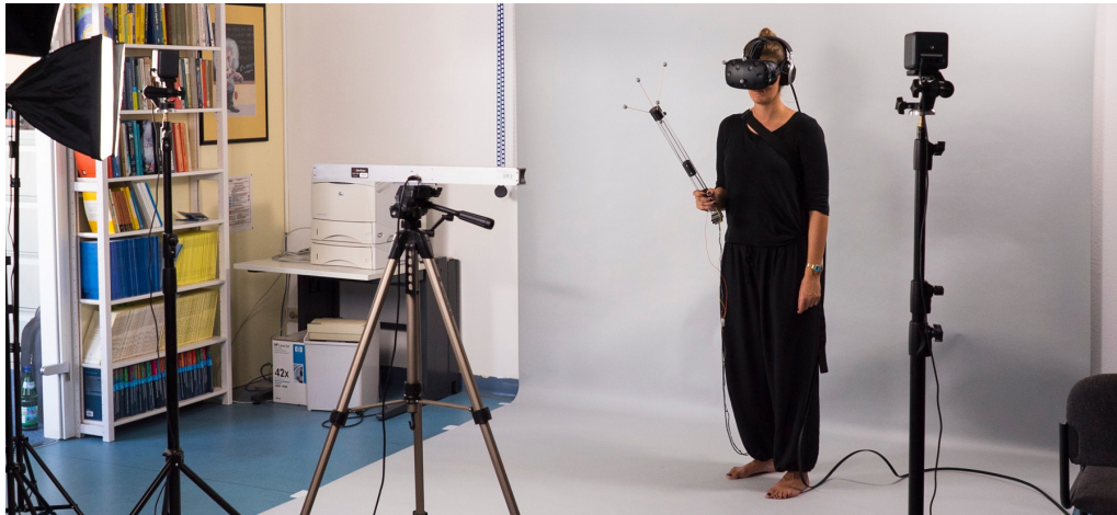
Figure 5.6: A user interacting with Shifty in our experiment setup. The user wears an HMD and headphones. The rigid-body target on the proxy is tracked by a motion capture system. © 2017 IEEE.
