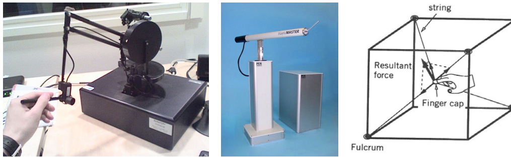
Figure 2.8: Three examples of world-grounded kinesthetic AHF. Left: PHANToM force feedback device [Massie and Salisbury, 1994] (Source: Wikimedia Commons; public domain 31 ). Center: HapticMaster (extracted from [Van der Linde et al., 2002]; © 2002 Van der Linde and co-authors). Right: SPIDAR system (extracted from [Sato, 2002]; © 2002 Sato).
