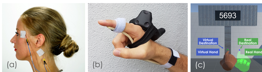
Figure 8.4: (a) Vibration cells at the temple and lower occipital regions close to the neck. (b) Finger splint and the HTC Vive Tracker used for hand tracking. (c) Vis-DT condition. Participants reach for the green target with the virtual hand while reading out the displayed number. Real hand added for illustration. All images © 2019 IEEE.
