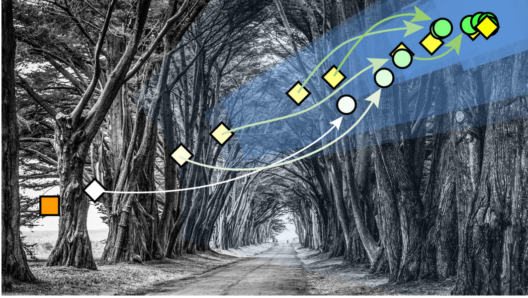
Figure 4.6. Gaze samples (yellow), landing position predictions (green) and corresponding prediction intervals (blue) for a sample saccade. The beginning of the saccade (orange), gaze samples and predictions are shown as the square, diamond and circular shapes, respectively. Color saturation level of the points indicates the time when each sample is observed and each prediction is made (more saturated color indicates more recent sample and prediction). Arrows connect gaze samples with our model’s corresponding predictions for the landing position.
