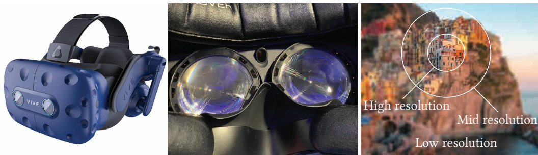
Figure 1.1. The HTC VIVE Pro Eye Headset 1 - a look from outside (left), and from the inside 2 (middle), showing the infrared LEDs used for eye tracking. The picture on the right presents an example of the traditional foveated rendering technique. [Guenter et al., 2012]
