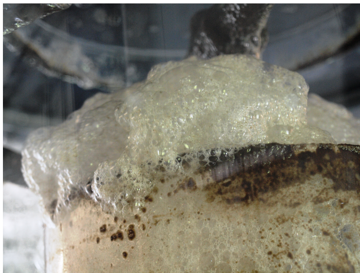
Figure 5. The upper part of a foam flotation where the foam is removed from the RAS. The brownish discoloration comes from particles and bacteria. A unique feature of foam flotation is that the filter medium, i.e., the bubble surface, is continuously replaced. The filter medium is air injected into a bubble column.
