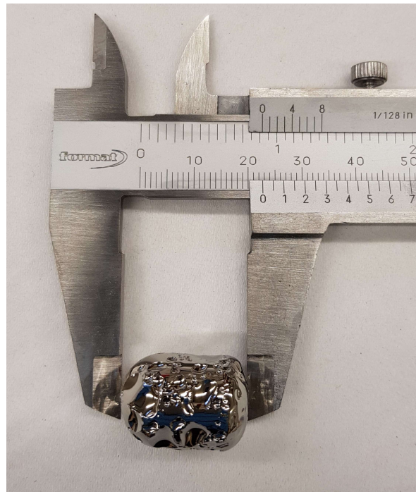
Figure 3-2: Purified Master-alloy of \text{Pt}_{42.5}\text{Cu}_{27}\text{Ni}_{9.5}\text{P}_{21} after the fluxing procedure with \text{B}_2\text{O}_3
