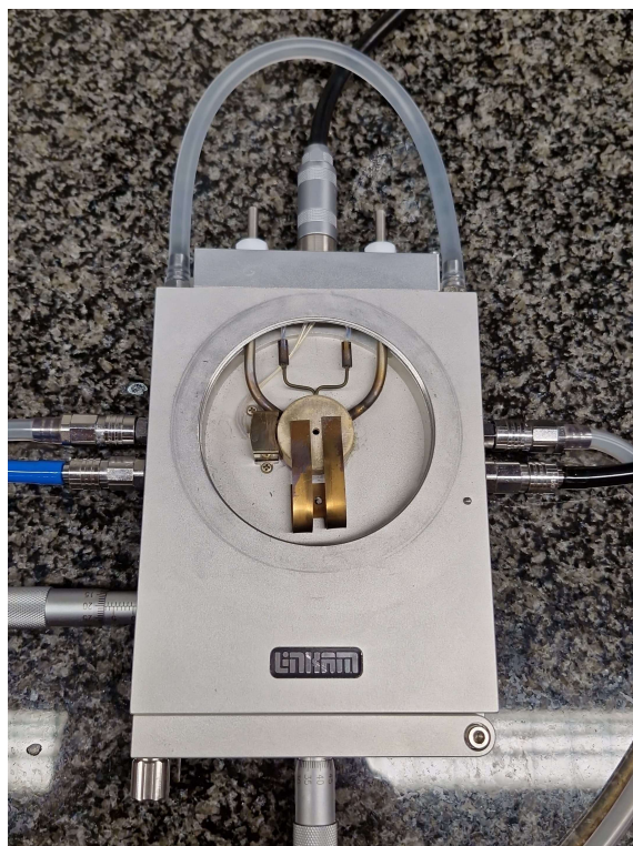
Figure 3-10: Linkam furnace THMS600 with the silver furnace within the chamber and the custom-built sample holder for the measurements in vertical position of the furnace. The side inlets and outlets are used for purge gas and a water-cooling of the chamber.
