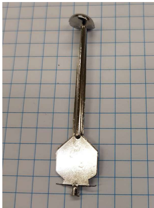
Figure 3-4: 0.5 mm thick plate out of Pt 42.5 Cu 27 Ni 9.5 P 21 with the 2 mm gate and cast-on section created through suction casting into an indirectly water-cooled Cu-mold.
