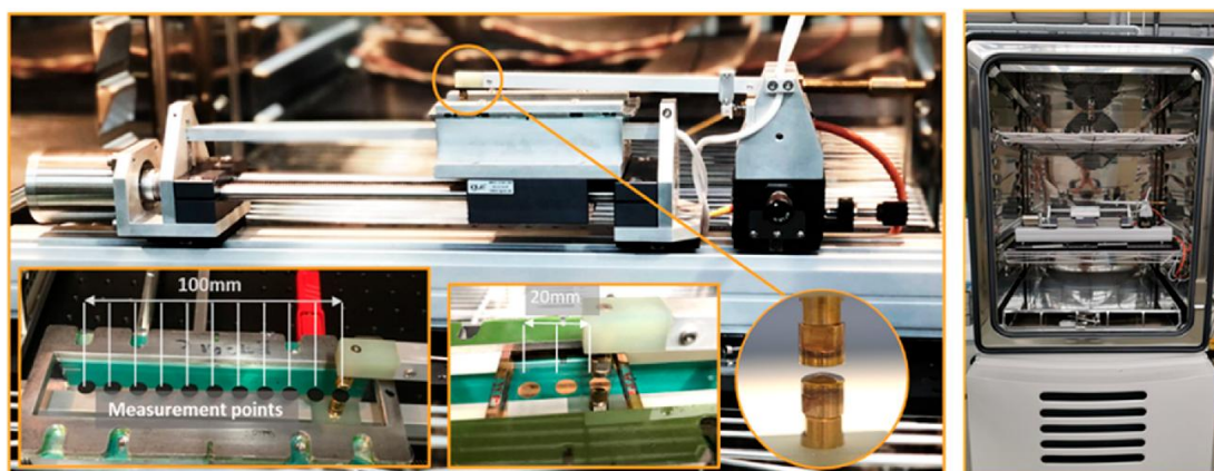
Figure 2. Left: Automated breakdown tester with measurement electrodes (convex/flat design for voltage application) and example of screen-printed and gold-sputtered electrodes. Right: Test setup in climate chamber CLIMEEVENT C/600/40/3, Fa. Vötsch.
