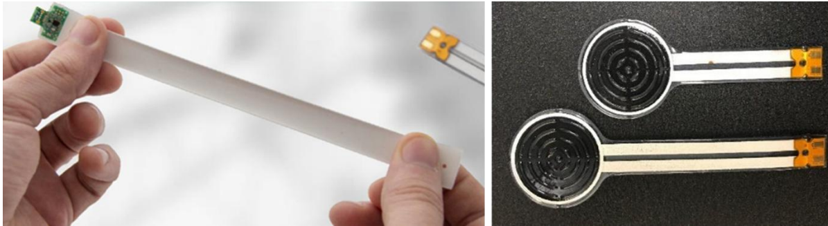
Figure 2.4. Stertch sensor for a respiration-monitoring functional shirt (left) and pressure sensor for gait analysis (right); kindly provided by IDEAS GmbH. Representative examples of both sensor types have been kindly provided by mateligen IDEAS GmbH.
