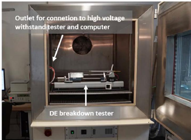
Figure 6. Placement of breakdown tester in climate chamber and outlet with connection to high voltage withstand tester, control unit and computer.
