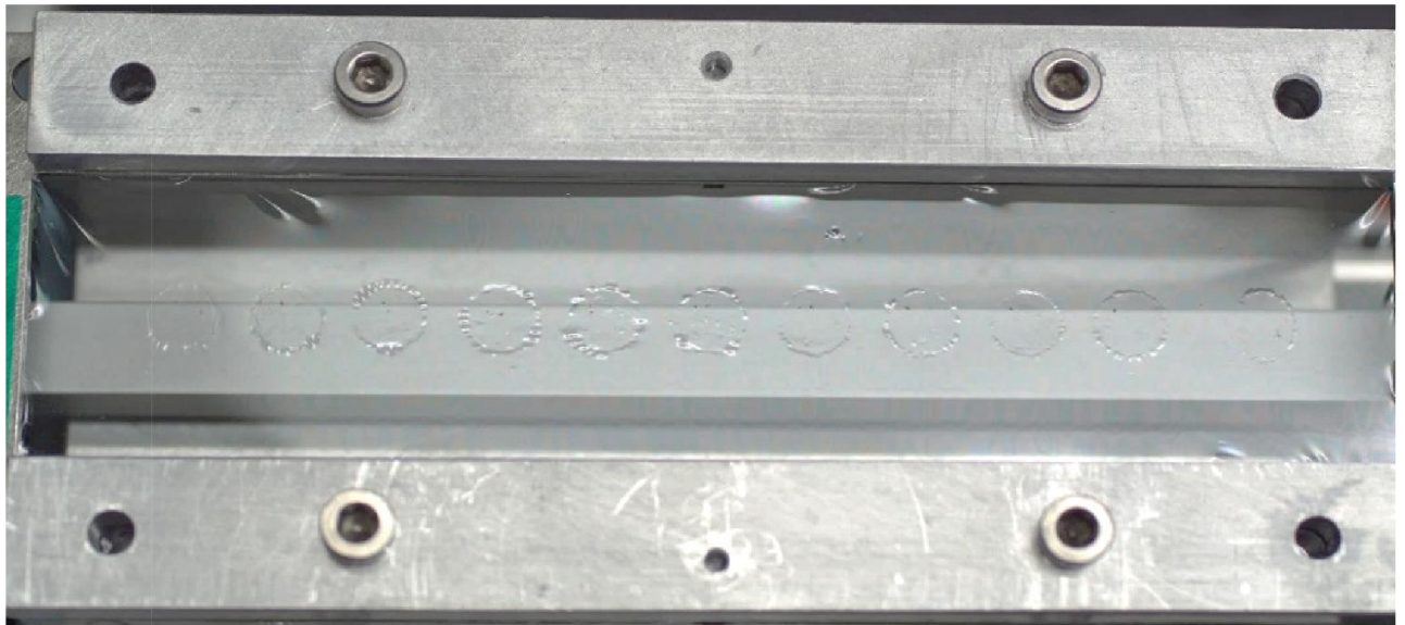
Figure 5. Dielectric elastomer film after dielectric breakdown test with circular flat electrode at eleven positions.
