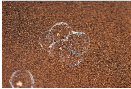
Figure 5.21. Example of multiple localized breakdowns and accumulation of repair pads
