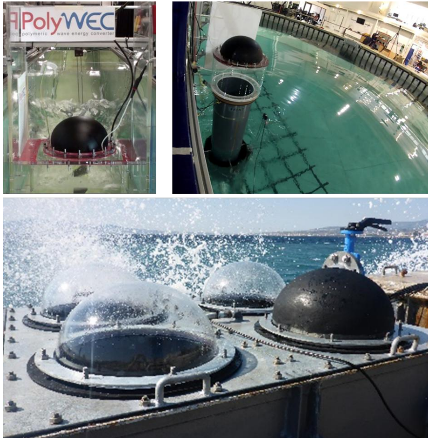
Figure 2.11. Pilot project of DEG for wave generator harvesting: DEG setup in pool using artificial wave energy (top), and DEG setup using wave energy from the ocean. Pictures courtesy from Giacomo Moretti.
