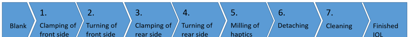
Figure 4. Machining steps for the production of customized IOLs.
